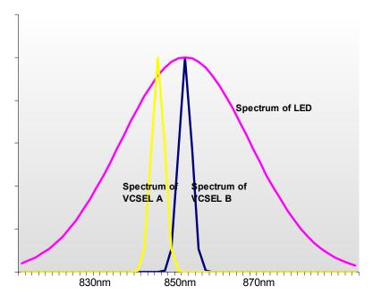
Fig 2: The spectrum of a VCSEL is narrow and different devices may have slight offset in the central wavelength. The spectrum of an LED, on the other hand, is much broader.
