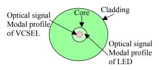
Fig 1: The optical signal from LED covers larger part of the fiber cross-section during the test, uncovering fiber formation defects
